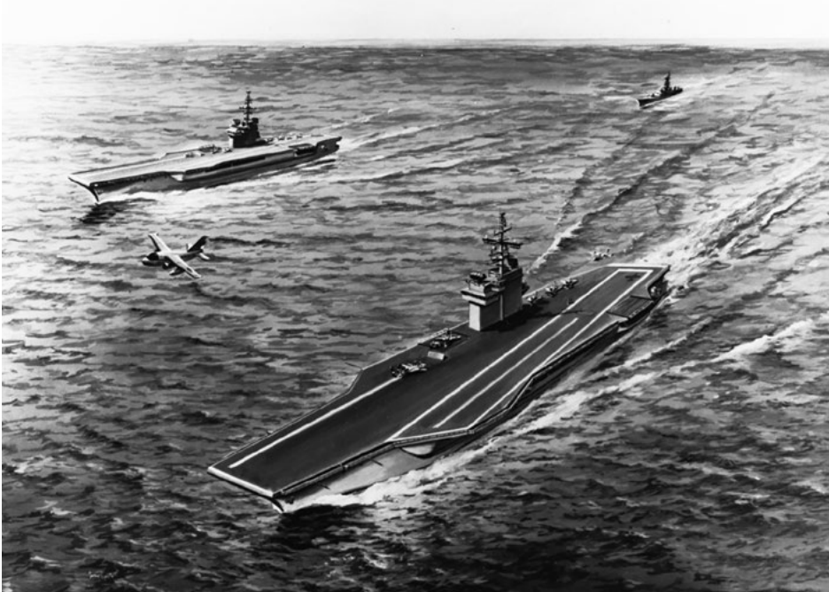
Artist's rendering of the Carter administration's version of the CVV—a replacement for the Midway -class carriers, capable of fielding VSTOL and conventional aircraft (NHHC/NH-88035).
